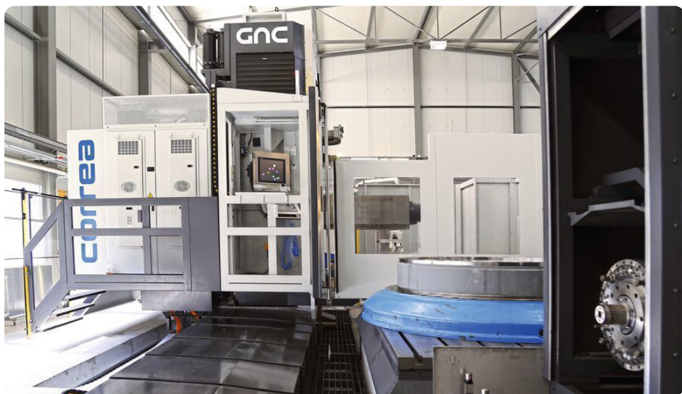
Hydro's milling machine AXIA is equipped with automatic head changer for two heads.
